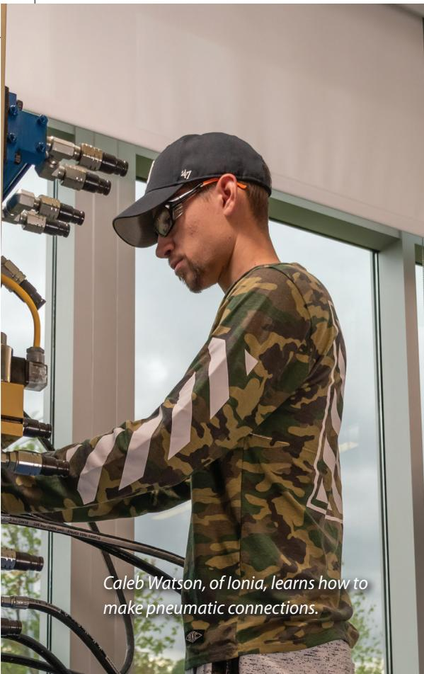
*Caleb Watson, of Ionia, learns how to make pneumatic connections.*
